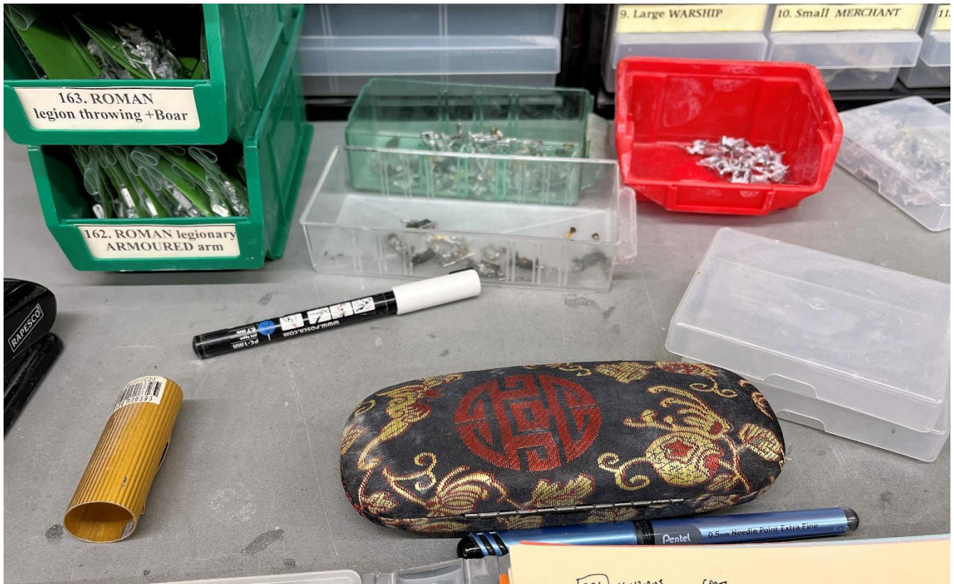
Small tray at back has the parts of the master figures after they are moved from the master mould. Green bins contain newest packs in production.
